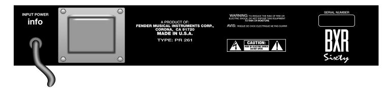
NOTE: DO NOT BLOCK THE AIR FLOW TO THE REAR PANEL, FOR EXAMPLE, BY BACKING THE AMPLIFIER UP AGAINST A WALL. The rear panel is used to keep the output devices from getting too hot. Should the amplifier overheat, a thermal switch will shut the amplifier off until the output devices cool.
